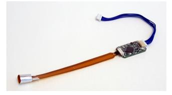
SKS1 is a temperature and relative humidity sensor adapted for UAV applications. The flexible arm that connects the sensor to the electronics makes it easy to place the sensor in undisturbed air and makes the sensor element itself replaceable. SKS1 is cheaper than SKS2 but has significantly slower response time.
