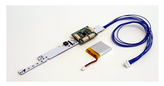
SKH1 is a hub for connecting sensors onboard UAVs. It synchronizes and provides power to all connected sensors. It also measures a basic set of parameters and provides logging and radio telemetry to a Sparv ground station.
