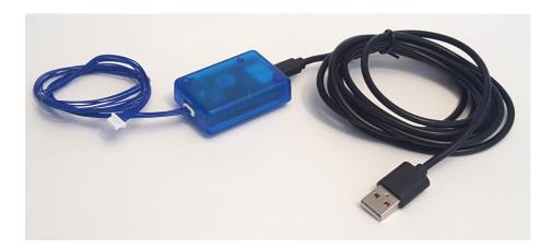
SA1 connects Sparvio to a computer for reading out log files. It only needs to be connected while reading logs, not during measurements. Use SA1 together with computer software.
